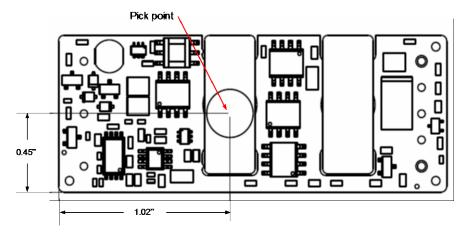
Fig. 3. Pick point of an eighth brick converter
