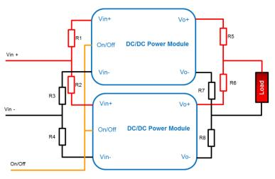
Figure 4 Power modules with droop current-share operating in parallel
