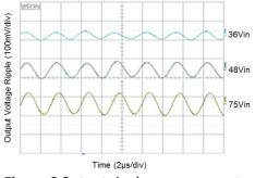
Figure 6 Output ripple measurement
