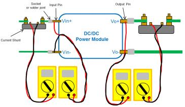
Figure 5 Efficiency measurement setup
