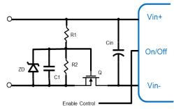
Figure 3 Typical Inrush Current Control Circuit
