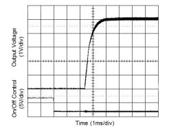
Figure 7 Output voltage monotonic startup
