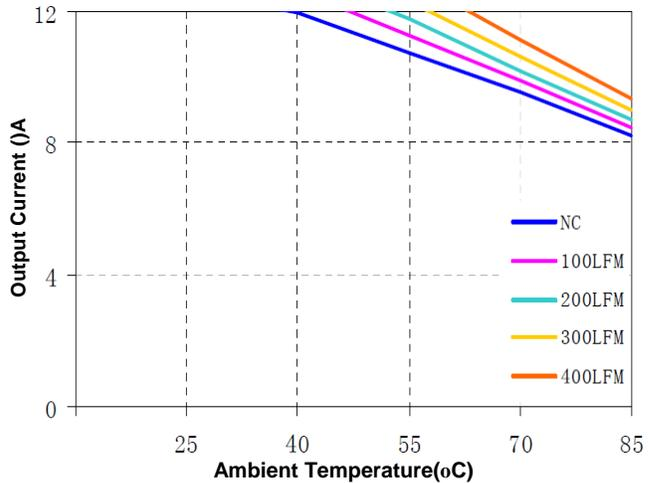
Figure 12(d) Current Derating Curve for 2.5V Output
