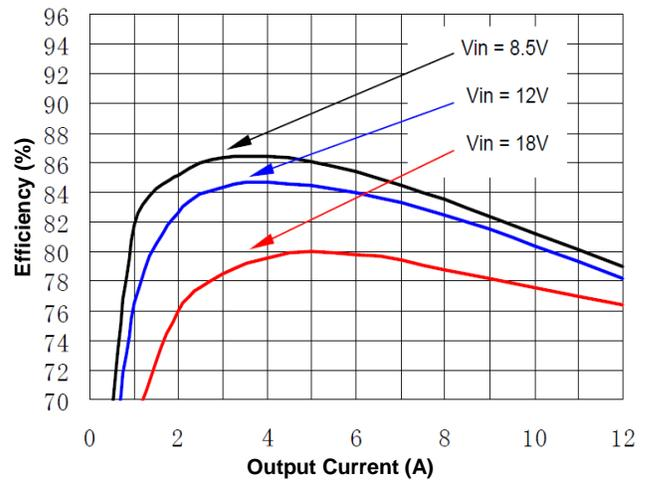
Figure 1(b). Efficiency vs. Load Current (25°C, 1V)
