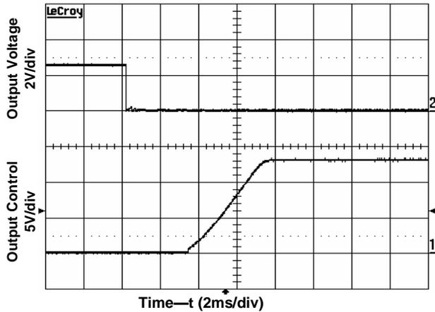
**Figure 4. Start-Up from Enable Control**
