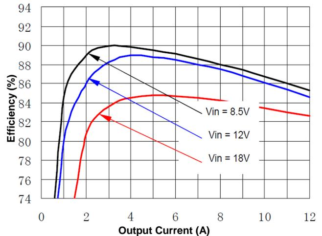
Figure 1(d). Efficiency vs. Load Current (25°C, 1.5V)
