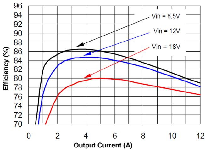
Figure 1(a). Efficiency vs. Load Current (25°C, 0.8V)
