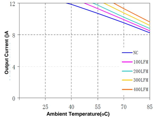
Figure 12(c) Current Derating Curve for 1.8V Output
