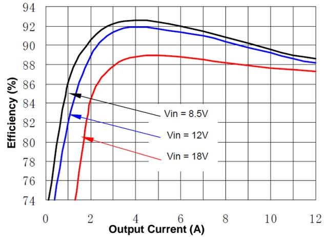
Figure 1(f). Efficiency vs. Load Current (25°C, 2.5V)
