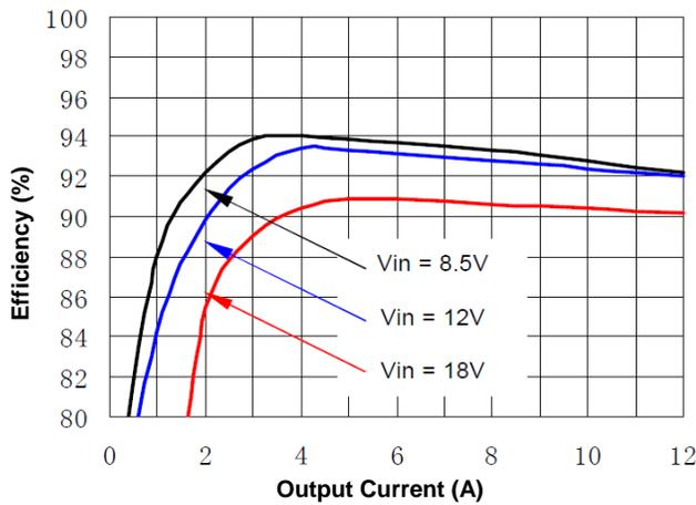
Figure 1(g). Efficiency vs. Load Current (25°C, 3.3V)
