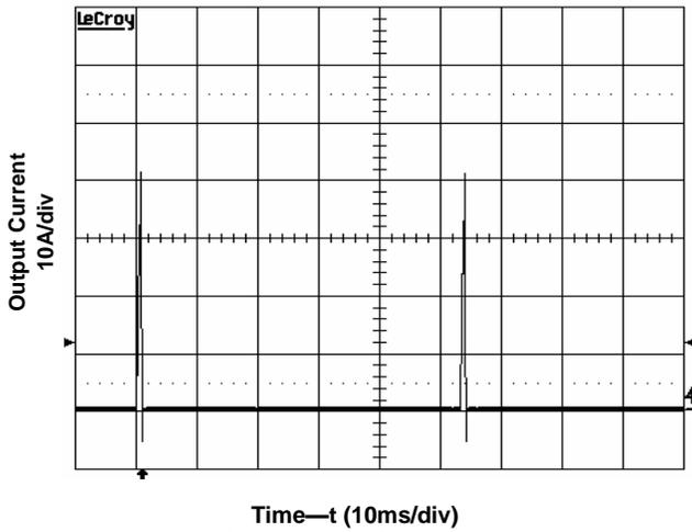
Figure 10 Short Circuit Current. Vin = 12V
