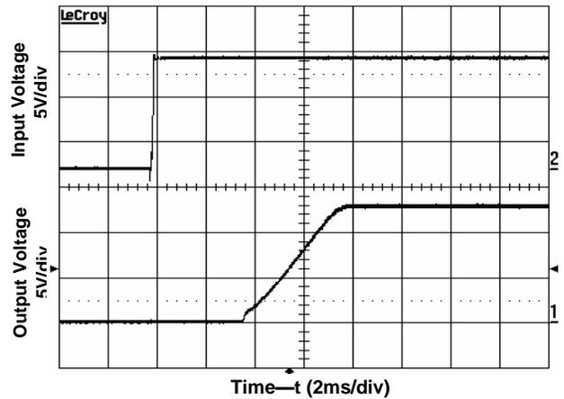
**Figure 5. Start-up Application of Input Voltage**
