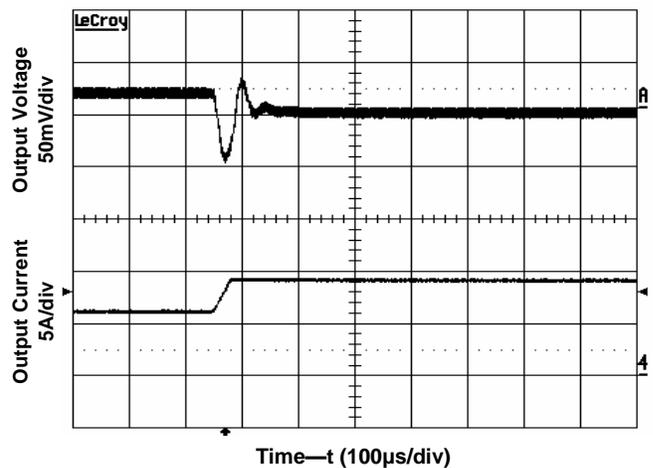
**Figure 9 Transient Load Response**
