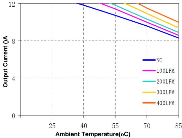
Figure 12(a) Current Derating Curve for 1.0V Output
