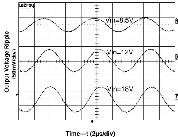
Figure 3. Output Reflected Ripple at 5V, 12A Output
