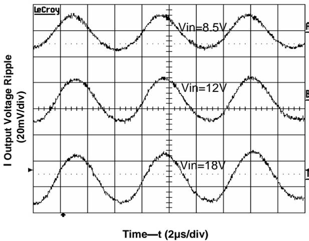
Figure 2. Output Voltage Ripple at 2.5V, 12A Output
