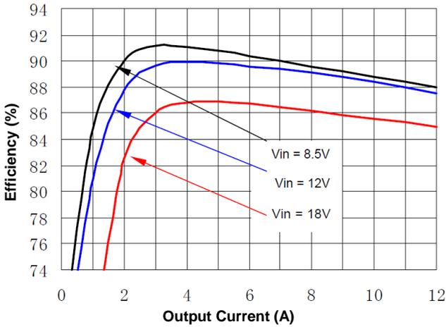
Figure 1(e). Efficiency vs. Load Current (25°C, 1.8V)
