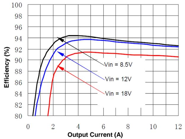
Figure 1(h). Efficiency vs. Load Current (25°C, 5V)
