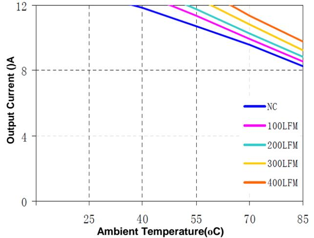
Figure 12(b) Current Derating Curve for 1.5V Output
