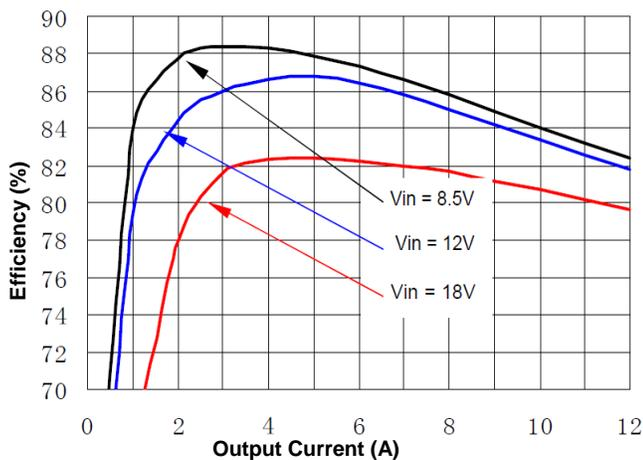
Figure 1(c). Efficiency vs. Load Current (25°C, 1.2V)
